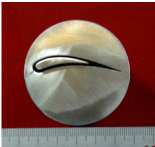
Fig. 5. Examples of casting mold and core for turbine nozzle. 7
